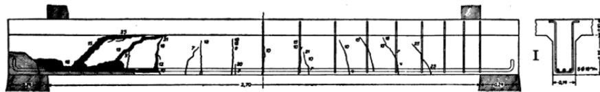
FIG. 131.—Beam I, 3 rods 18 mm. diameter, breaking load, 25.7 t. (27.3 tons).
